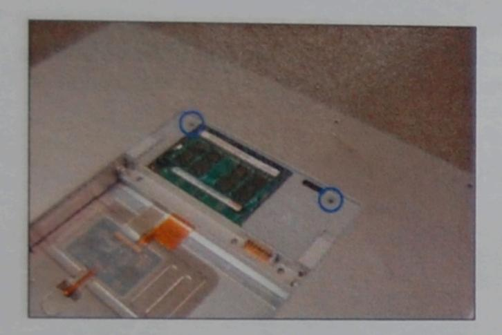
Remove two Torx T6 screws, shown circled in blue, from rear of memory compartment.
